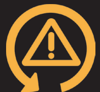
Traction Control Fault Light
