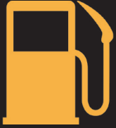
Fuel Warning Light
